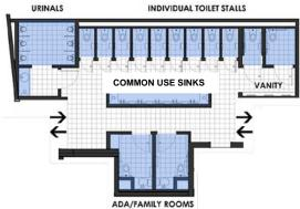
This design features stalls that can be designated All Gender with floor to ceiling doors. In addition, common use sinks/open hand washing station is available to all users. ADA/Family restrooms and urinals are also a feature.
