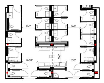
2. GATE C2/3 – Convert one set of restrooms to single-user All Gender Restrooms using the recommended compartment-style design. This could mean up to six (6) compartments at Gate C2/3. The signage will be gendered (male or female) to accommodate the current building code requirements. The gendered signage can be replaced in the future to the recommended All Gender signage once building code is updated.
