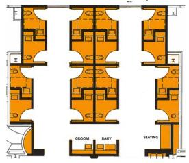
This design features compartments where toilet and sink are in one enclosed private space with floor to ceiling doors.
