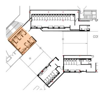
3. GATE D3 — Convert one set of restrooms to single-user All Gender Restrooms using the recommended compartment-style design. This could mean up to nine (9) compartments. The signage will be gendered (male or female) to accommodate the current building code requirements. The gendered signage can be replaced in the future to the recommended All Gender signage once building code is updated.
